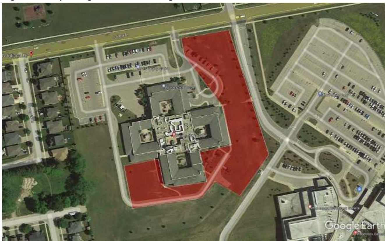
Figure 2 – Proposed ground heat exchanger bore field area.
