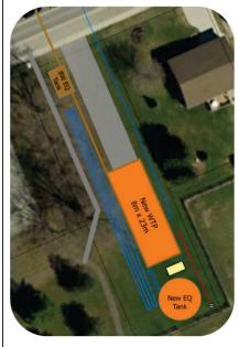
Alternative 6a/b: Two-Stage Pumping with on-ground storage, iron and manganese filtration, and split-stream or full stream IX treatment
