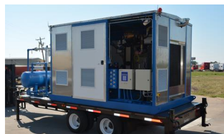
Figure 46 Mobile CNG Fueling Compressor Station
