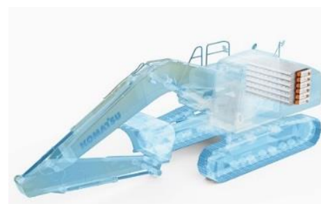
Figure 30 Rendering of Komatsu Battery Electric Backhoe
