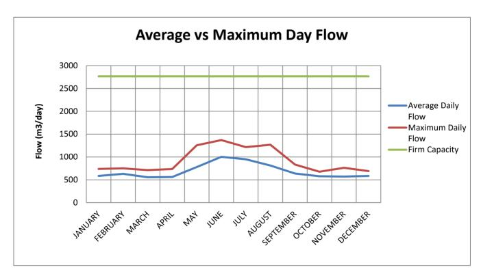
Thamesford Water System Supply Capacity 5,391 m³/day Thamesford Water System Firm Capacity 2,765 m³/day
