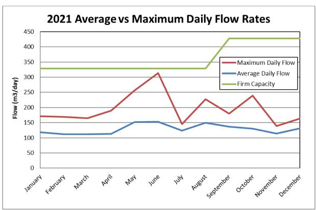
Mount Elgin Water System Supply Capacity 1,192m³/day Mount Elgin Water System Firm Capacity 428 m³/day
