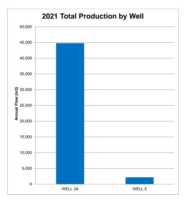
Mount Elgin Water System Supply Capacity 1,192m³/day Mount Elgin Water System Firm Capacity 428 m³/day
