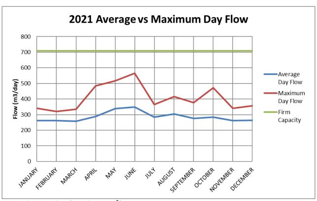
Drumbo-Princeton Firm Capacity 709 m<sup>3</sup>/day Drumbo-Princeton Water Supply Capacity 1,329 m<sup>3</sup>/day
