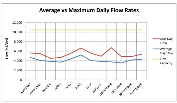
Ingersoll Water System Supply Capacity 17,357 m<sup>3</sup>/day Ingersoll Water System Firm Capacity 10,454 m<sup>3</sup>/day
