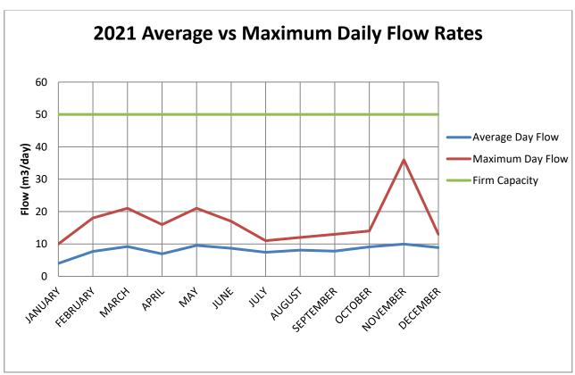
Dereham Centre Firm Capacity 50 m³/day Dereham Centre Water Supply Capacity 50 m³ /day
