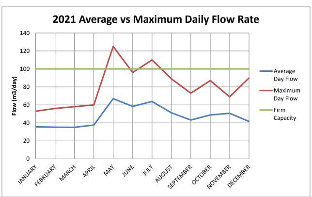
Lakeside Firm Capacity is 100 m³/day Lakeside Water System Capacity 270 m³ /day
